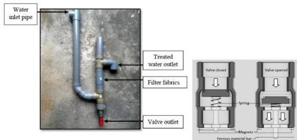
Fig. 5. Schematic of a rainwater filtration system Left figure adopted from Ref. [8] Right figure adopted from Ref [9]
