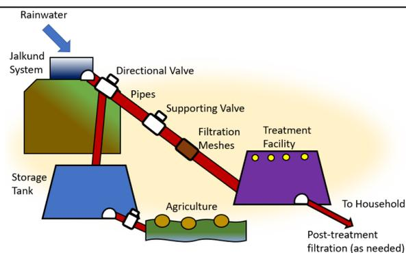
Figure 6, Jalkund and water treatment system design for this project.
