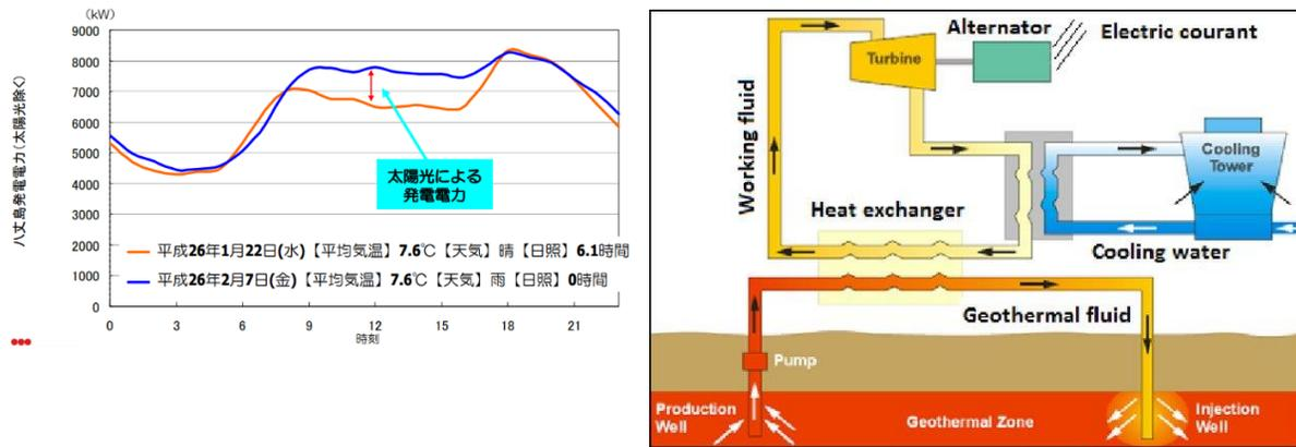
Figure 2. (Left) Energy demand (solar power excluded) in Hachijojima at various hours of the day. Adopted from [cite] (Right) Schematic of a binary geothermal power plant
