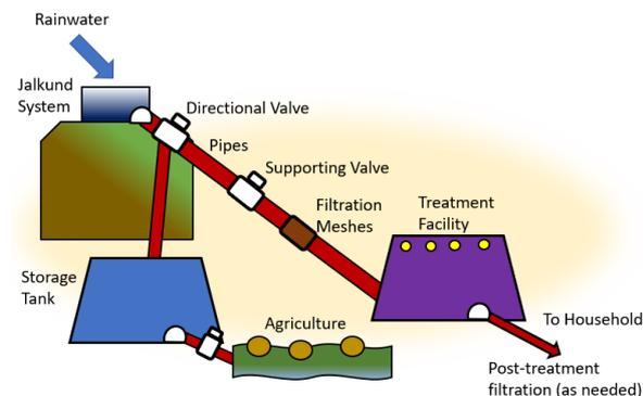
Fig. 7 Schematic of the Jalkund-based water collection, distribution, and purification system
