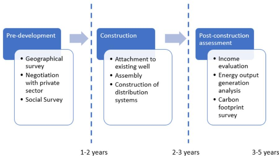
**Figure 2.** Proposed timeline for construction of binary geothermal plant for existing wells.
