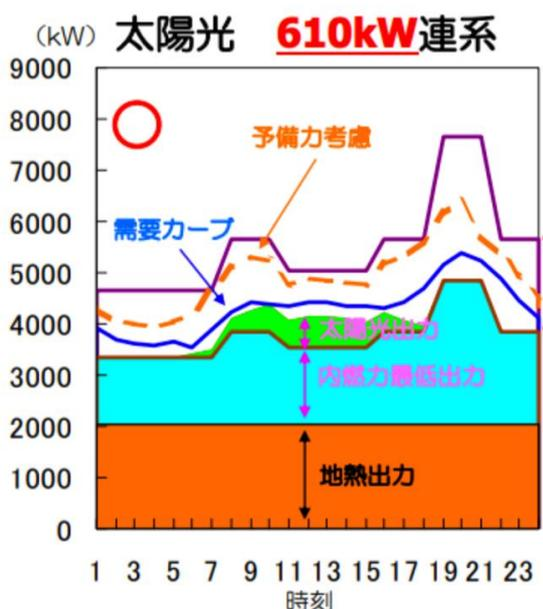
Figure 2. Graph showing the fluctuating demand on the island throughout the day and indicating baseload supply delivered by geothermal (orange) and diesel combustion (cyan). Source TEPCO 2014
