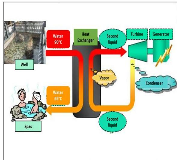
Figure 4. Diagram of a binary geothermal power plant combining Onsen with power generation. Image source: Movellan 2015.
